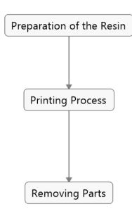
The material should be processed at room temperature. Before usage the material should be shaken well. Pour it slowly in the vat and wait a couple minutes, until smooth, bubble-free surface is obtained before starting the print job.
